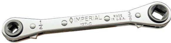
**127-C** Compressor access valve wrench. Chrome plated. Has 1/4", 3/8", 3/16" and 5/16" square drive ratchets and is specifically designed for use on compressors with access valves in hard to reach places. Reversible ratchets.
