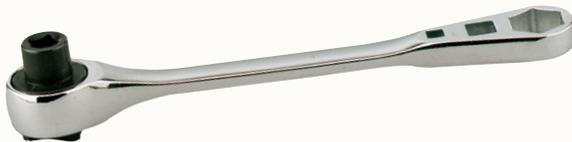
**125-C** Rugged steel forged wrench with four sizes covering almost any application. Ratchet has 1/4" square drive on one end, other end has 3/16" and 5/16" square openings, plus 9/16" hex opening.
